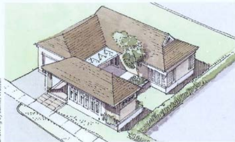
7-9. A detached outbuilding is built in the front yard, creating a private interior courtyard and preventing the garage and driveway from dominating the street view
