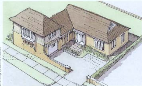
7-7. The existing garage is converted into additional living space as a two-story structure built over the existing driveway
