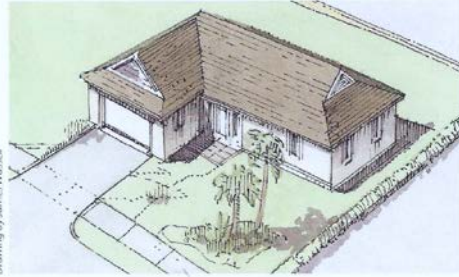
7-6. The existing condition is an excessive front setback dominated by a driveway and a parking garage
