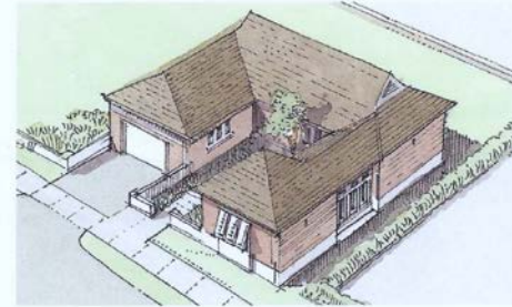
7-8. A new wing is added, creating an entry courtyard and preventing the garage and driveway from dominating the street view
