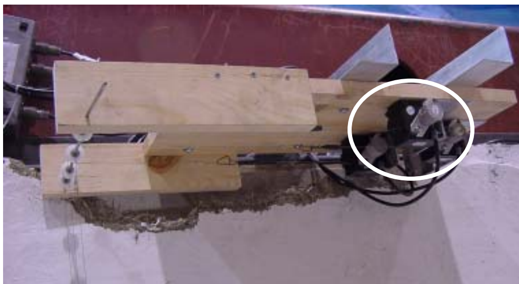
Figure 5.4 – Cable-extension transducer array photograph (transducer circled)
