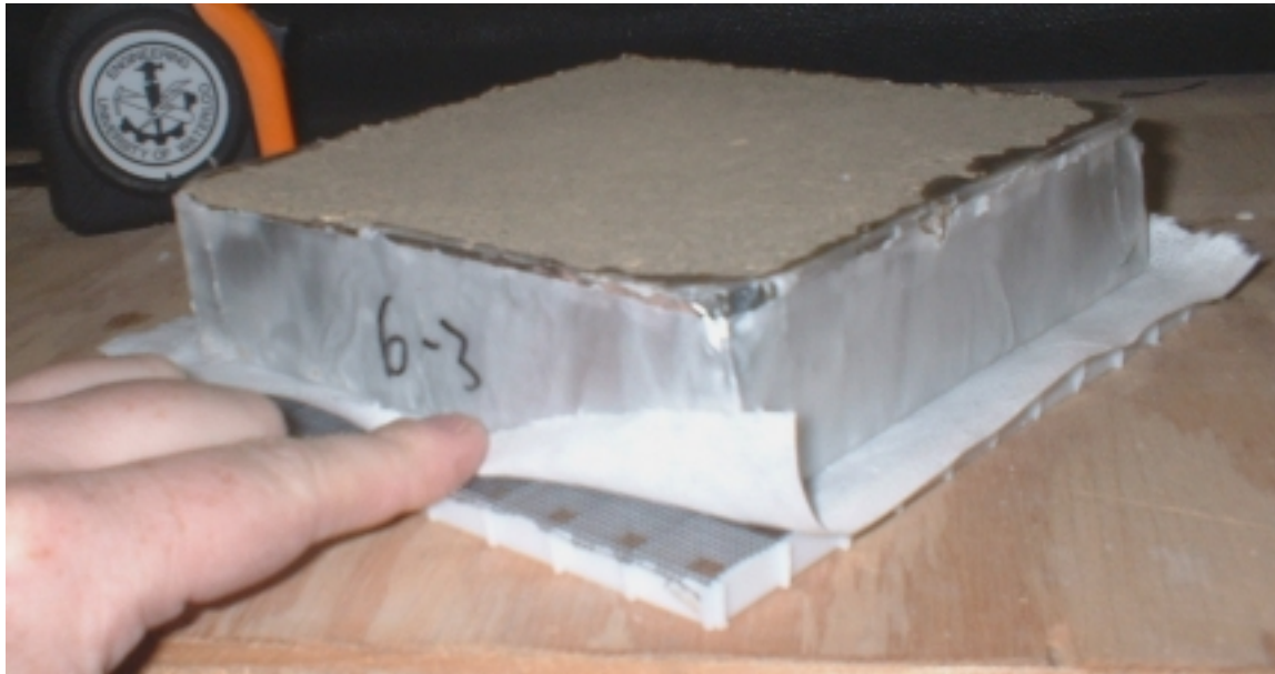
Figure 5.2: Sample preparation for water absorption test
